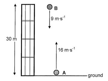
3.3 Calculate how high above the ground ball **A** will be at the instant the two balls pass each other.
