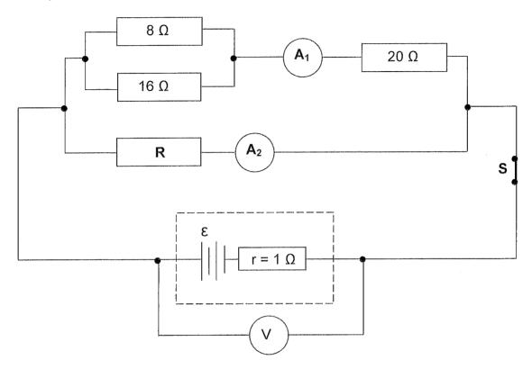
With switch  $\bf S$  closed, the current passing through the 8  $\Omega$  resistor is 0,5 A.
