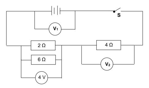
When switch  $\mathbf{S}$  is closed briefly, the potential difference across the parallel combination is 4 V.
