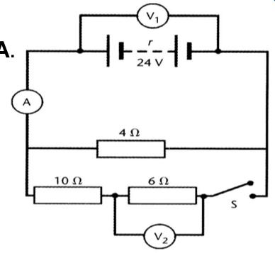
V<sub>//</sub> = V<sub>1</sub> and this p.d. is divided between the 10 Ω and 6 Ω resistors (they are in series with one another) in the proportion 10 : 6 or 5+3. The 6 Ω resistor will draw **less** = 7,8 ∨ energy from the current, therefore
