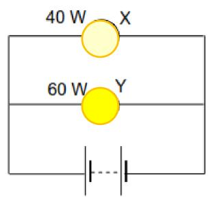
Bulb Y glows brighter than bulb X.
