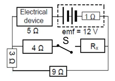
$R_{tot}$  will increase since all resistors are now in series  $\Rightarrow I_{tot}$  will decrease and therefore  $P_{device}$  will decrease. No, the device will no longer function at maximum power.
