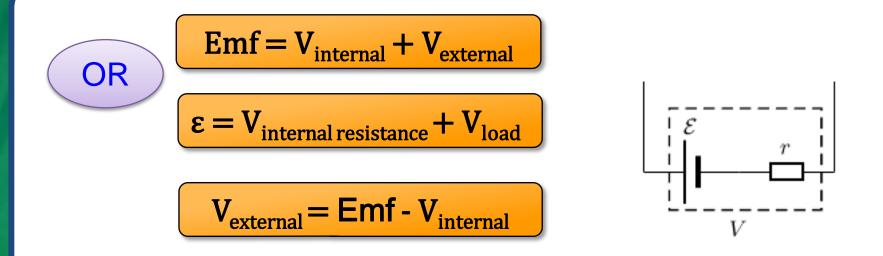
emf = terminal potential difference + "lost volts" Emf = IR + Ir = I(R + r)
