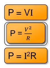
The rate of energy transfer to a resistance is directly proportional to  $I^{(2)}$
