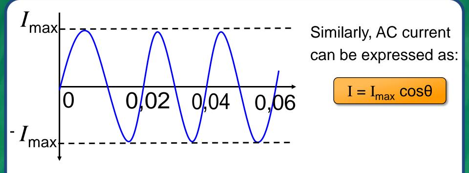
The current generated **fluctuates** between  $+I_{max}$  and  $-I_{max}$ , with smaller + and - values in between. The **average value** of the current for one cycle is zero.
