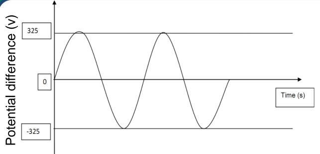
3. The waveform is a graphical representation of the variation of voltage (V) vs time (t) for an AC current.
