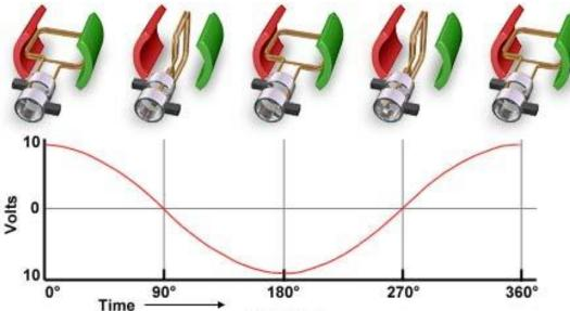
A coil cutting through a basic magnetic field in a clockwise direction will at first result in a emf with positive polarity, but as it cuts across the same field in the opposite direction during the second half of its turn, the polarity becomes negative. Note the **slip rings** – slip rings identify a generator or motor **as AC** rather than DC
