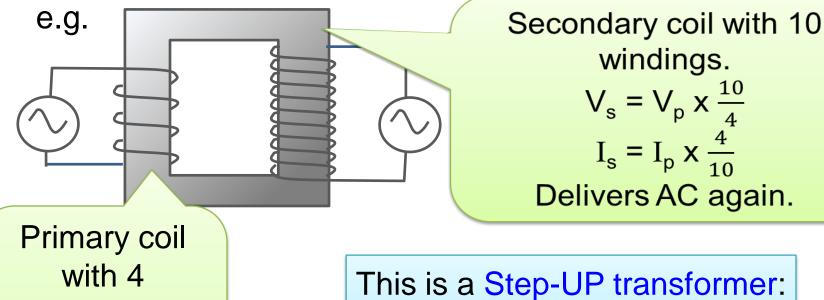
This is a Step-UP transformer: While voltage is **increased**, current is **de**creased.
