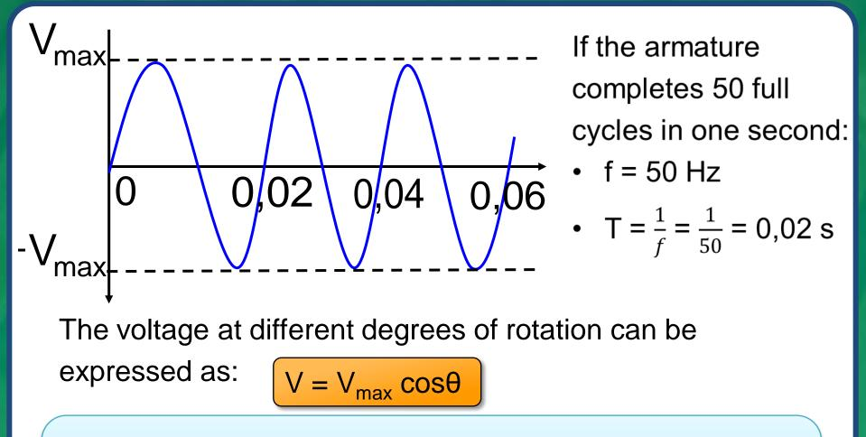
Note that the voltage generated **fluctuates** between  $+V_{max}$ and  $-V_{max}$ , with smaller + and – values in between. The **average value** of the voltage for one cycle is zero.
