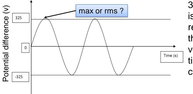
3. The waveform is a graphical representation of the variation of voltage (V) vs time (t) for an AC current.
