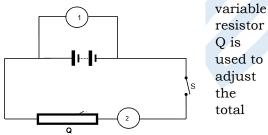
resistance of the circuit. In order to take the readings, the switch is closed for a SHORT PERIOD. The switch is then opened.
