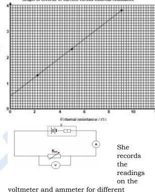
voltmeter and ammeter for different resistances of the rheostat. The graph below was obtained from the results.
