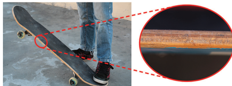
Figure 23: A skateboard is made of plywood
