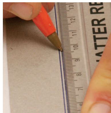
Figure 19: Make a fold by first making two grooves on the inside.
