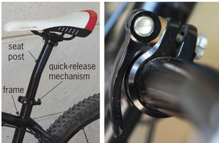
Figure 12: A quick-release mechanism is used to clamp the seat post to the frame of this bicycle.
