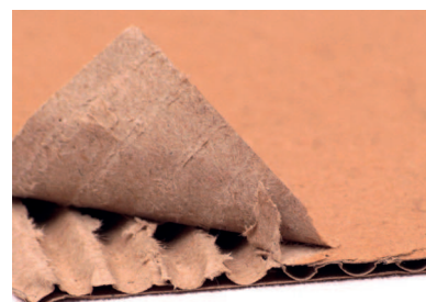
Figure 11: Large boxes are made of corrugated cardboard.
