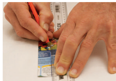
Figure 18: Make a fold by first making a groove on the outside.
