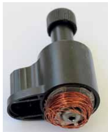
Figure 5: The exposed copper coils in a dynamo
