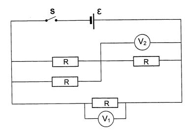
When switch  ${\bf S}$  is CLOSED, the reading on voltmeter  $V_1$  is 3 V.
