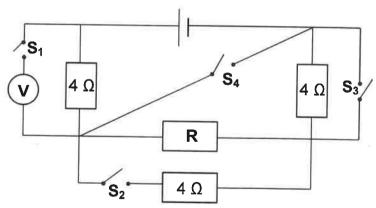
Which ONE of the switches must be closed to increase the power in resistor  ${\bf R}$  the most?
