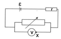
The circuit diagram consists of a cell with emf  $\epsilon$  and resistor r. A voltmeter is connected over a variable resistor that can be set to *known values* R.
