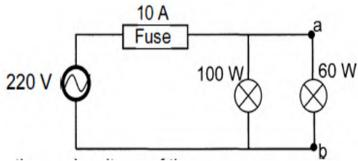
Two light bulbs rated at 100 W; 220 V and 60 W; 220 V respectively are connected to an AC source of rms value 220 V. The fuse in the circuit can allow a maximum current of 10 A. Ignore the resistance of the conducting wires
