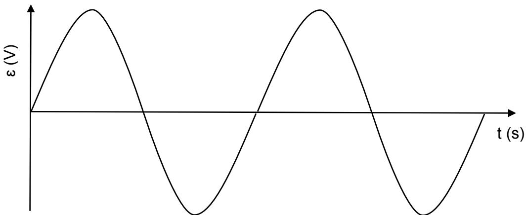
The speed of rotation of the generator's coil is now DOUBLED. What happens to the emf and the period of one cycle?
