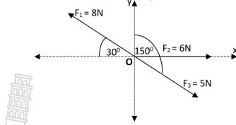
Three forces  $F_1$ ,  $F_2$  and  $F_3$  act at a common point O as shown in the diagram above.
