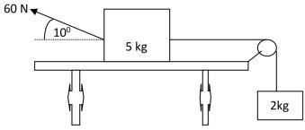
The coefficient of kinetic friction between the 5 kg block and the surface of the table is 0.5. Ignore the effects of air friction.
