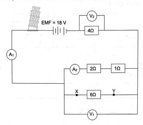
180 C of charge passes through the  $2\Omega$  resistor in 1,5 minutes.
