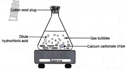
The cotton wool plug placed in the mouth of the flask prevents spillage of reactants and products, while simultaneously allowing the formed gas to escape. The balanced equation for the reaction that takes place is:
