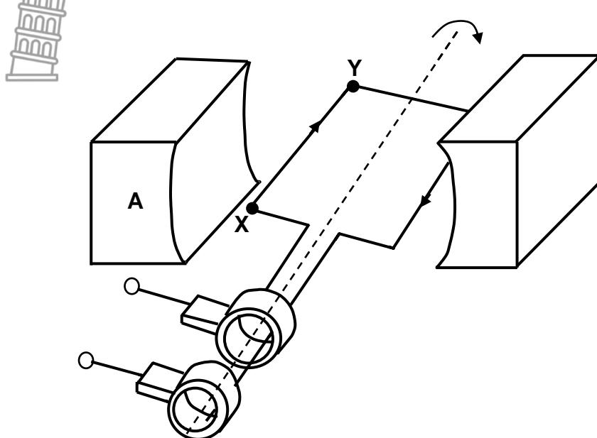
When the coil of the generator rotates clockwise between the two poles of the magnet, the direction of the induced current is from **X** to **Y**, as shown above.
