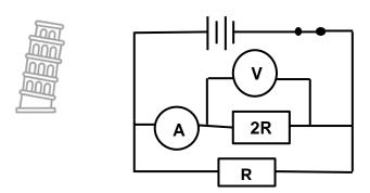
The current in the circuit is **I**. What are the readings on the ammeter and voltmeter?
