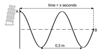
The frequency of the wave is 2,5 Hz.
