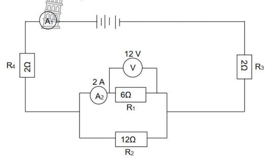
The voltmeter reads 12 V, while ammeter A2 reads 2 A.
