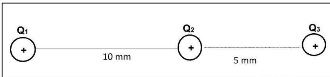
Calculate the net electrostatic force experienced by point charge **Q<sub>3</sub>** due to point charge **Q<sub>1</sub>** and **Q<sub>2</sub>**.
