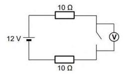
What will be the reading on the voltmeter V?
