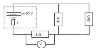
A voltmeter connected across the 8  $\Omega$  resistor reads 21,84 V. Calculate the:
