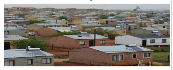
In areas of South Africa where electricity had traditionally not yet been provided, state subsidized solar panels and solar powered hot water cylinders have been installed on houses to harness the power of the sun to electricity houses.
