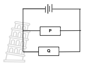
The resistance of conductor **Q** is much greater than that of conductor **P**. How does the potential difference across conductor **Q** and the current in **Q** compare to that of conductor P?
