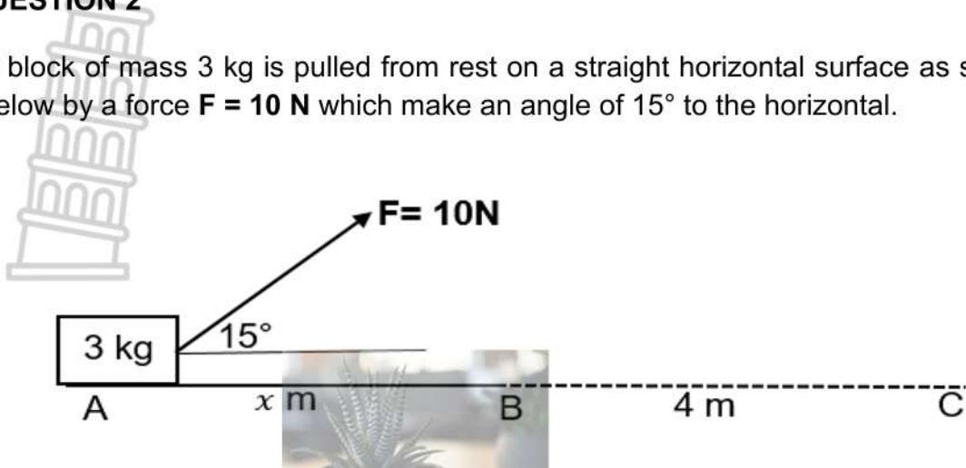
Path **AB** is  $x \text{ m}$  and is frictionless and path **BC** is 4 m and is rough. The coefficient of kinetic friction between the block and the surface **BC** is 0,53. The block comes to rest at point **C**.
